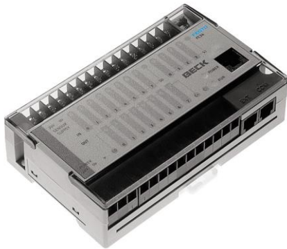
Figure 7.3 : automate programmable industriel (Sté Festo)
