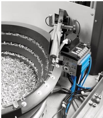
Figure 4.1: Vibration feeder for storing and sorting screws
