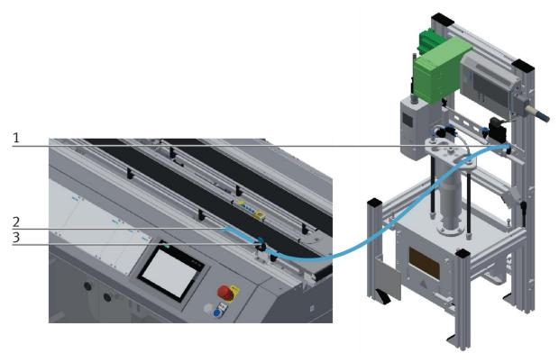
Pneumatically connect application module / illustration similar
