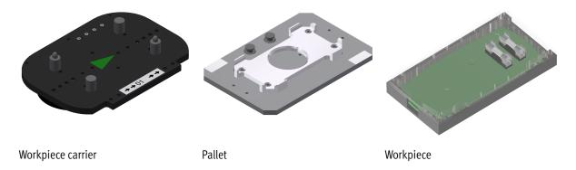
Workpiece carriers are transported on the base module conveyors. Pallets with fixed workpiece holders are placed on the workpiece carriers. The workpieces are placed on the workpiece holder or removed from there. In some stations, pallets can also be placed on a workpiece carrier or picked up from there.
