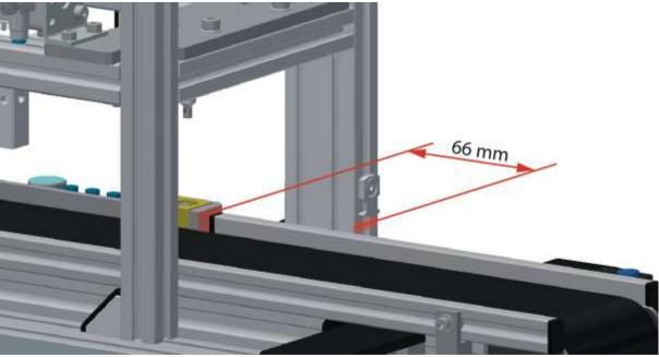
$\label{prop:equation} \textbf{Example distance between application module and stopper / illustration similar}$
