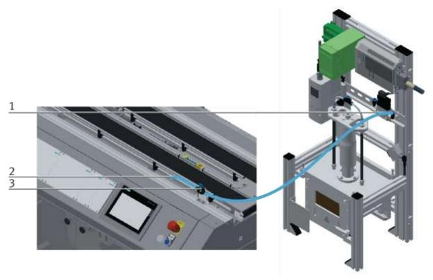
Pneumatically connect application module / illustration similar
