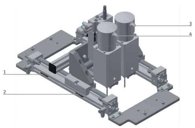
Sensors x-axis / drilling machines / illustration similar
