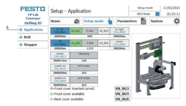
5. Application is selected to set up the application module. The corresponding actuators can be started by pressing the buttons. All other areas are for display purposes and cannot be influenced.
