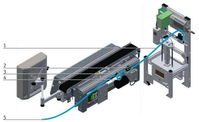
Pneumatically connect application module / illustration similar
