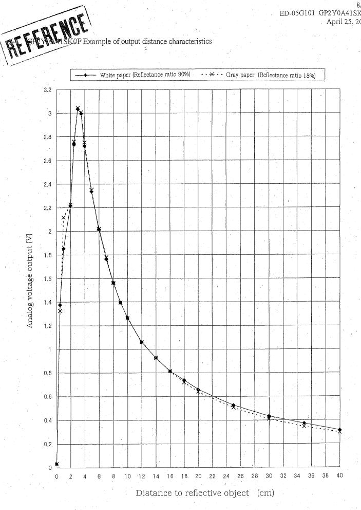
Example of output distance characteristics with the inverse of distance
