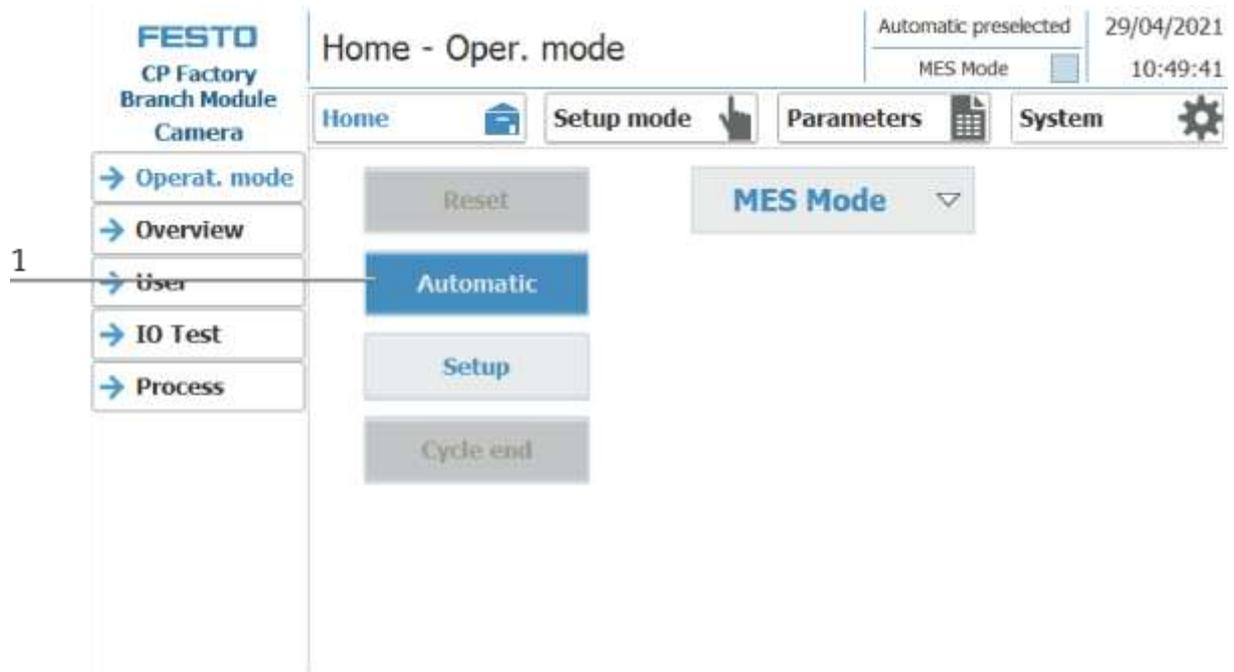
2. Automatic button flashing blue – Press Button to activate operation mode automatic
