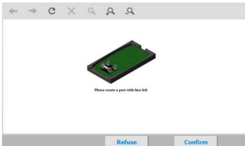
3. In this case, the html page was designed so that a work instruction for mounting the front fuse appears in the worker's guidance.
