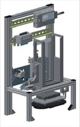
5. Application is selected to setup the application module. The corresponding actuators can be started by pressing the buttons. The sensors are only for display and cannot be set manually
