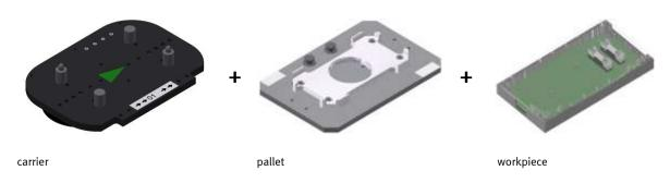
Carriers are transported on the conveyors of the basic modules. And on the carriers, there are pallets with a fixed workpiece reception placed. The workpieces are placed on the workpiece reception or taken from it. Pallets can also be placed on a carrier in some stations or gripped from there.
