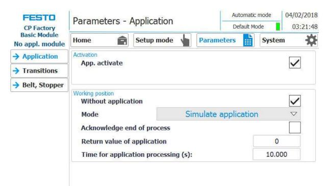
1. If the mode is simulate application and a carrier moves into the application, it is stopped. The application procedure is simulated, this is indicated by the following screen.
