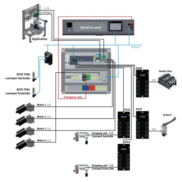
Cabling chart frontside siemens controller / illustration similar
