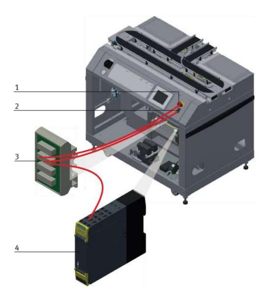
Structure of the emergency- stop system example / illustration similar
