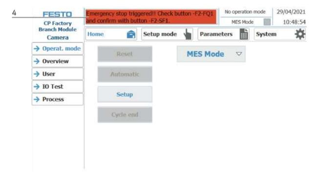
5. The error message is displayed in the main window. After the error situation has been remedied, it can be acknowledged by pressing the RESET button.
