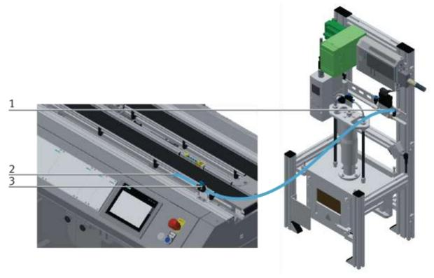
Pneumatically connect application module / illustration similar
