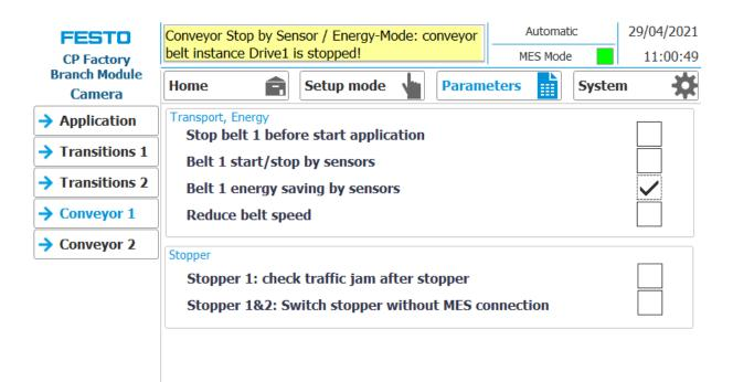
If the belt energy saving by sensors function is activated and the belts stop when there are no workpiece carriers on the belt, this is displayed in the upper message window.
