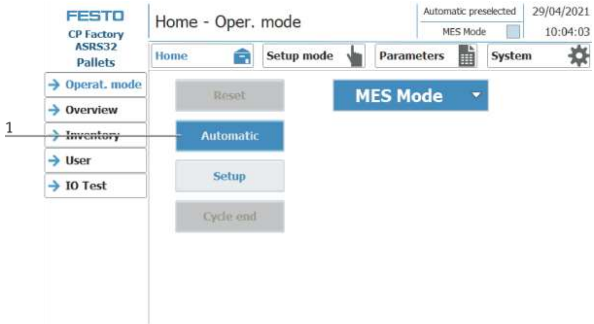
1. Automatic button flashing blue – Press Button to activate operation mode automatic
