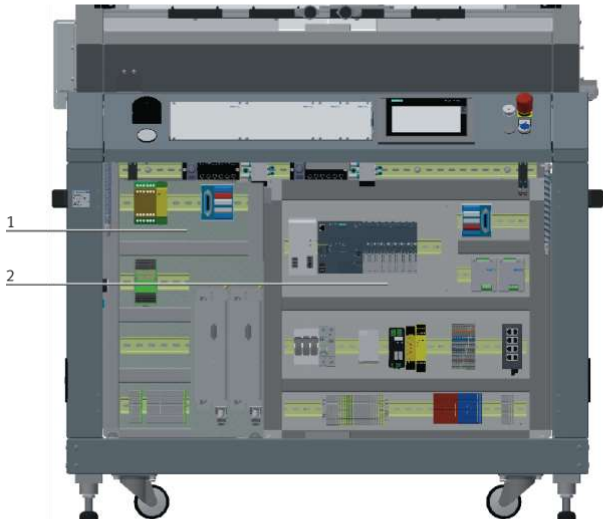
Electric boards ASRS for pallets example / illustration similar
