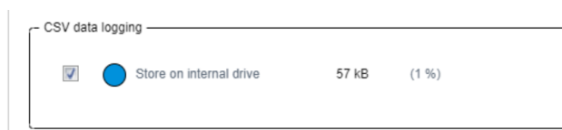
Figure: Activated data recording to the internal memory
